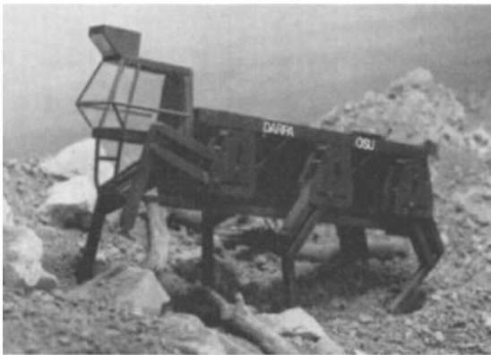
FIGURE 47.4 The adaptive suspension vehicle ( \frac{1}{10} -scale model). This is a vehicle for transportation in very rough terrain conditions which uses legged locomotion. ( The Ohio State University. )
